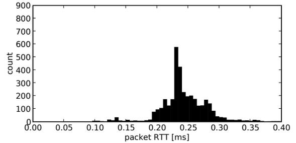
(b) RTTs between a hardware virtualized Linux VH and a simulation
